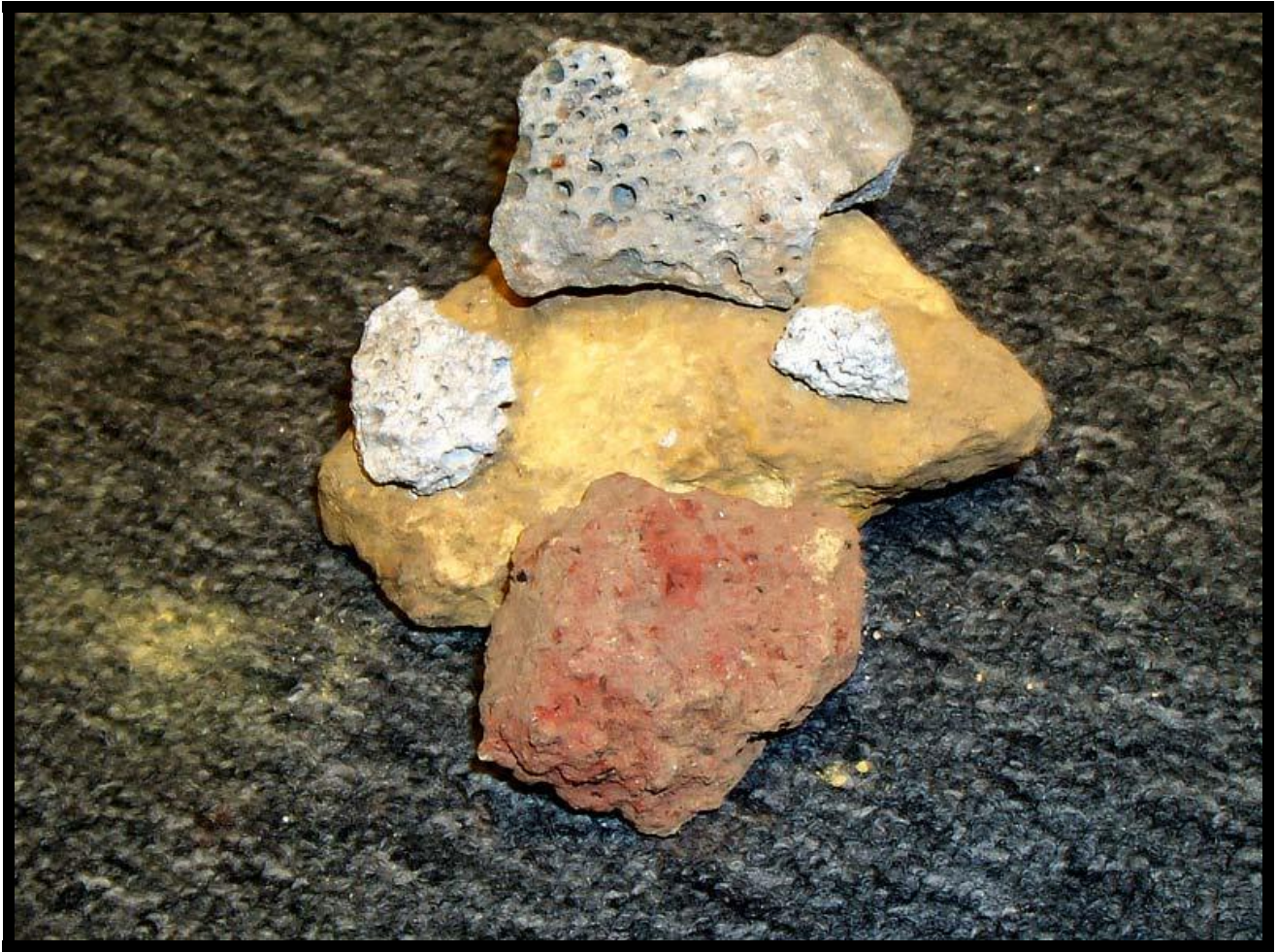
Typical view of slag fill at the Port of Rochester.
